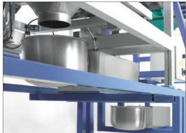
HAVER CPA 4 GRAVIOPT with two Revolving Hopper Scales for the sieve overflow and sieve underflow
