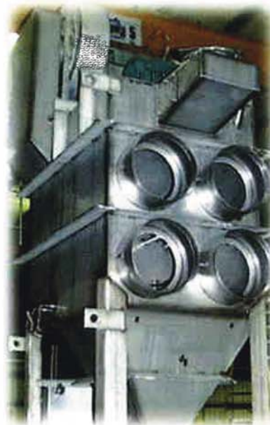
Cartridge Collector with "Bag-In/Bag-Out" feature
