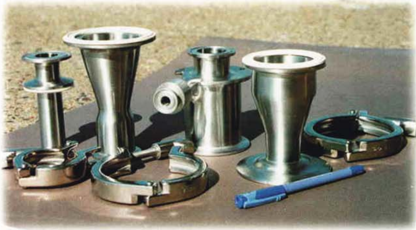
Break-apart cyclone disassembled for cleaning
